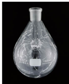
Coating glass breakage test
