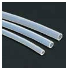
This tubing is made of materials specially formulated for peristaltic pumps and is highly durable. Sizes are checked for each lot, and those that meet the standards are carefully selected. The tubing withstands repeated autoclaving and has passed the standards for silicone rubber, including an elution test. Heat resistance temperature is up to 200°C.
