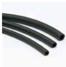
This tubing has excellent chemical resistance and is the most corrosion resistant of the four types of tubing. This high grade tubing is made of a base of fluororubber and can be used in highly corrosive solutions. Compared to standard Viton® tubing, it has superior physical strength, ozone resistance, and weather resistance. Heat resistance temperature is up to 204°C.
